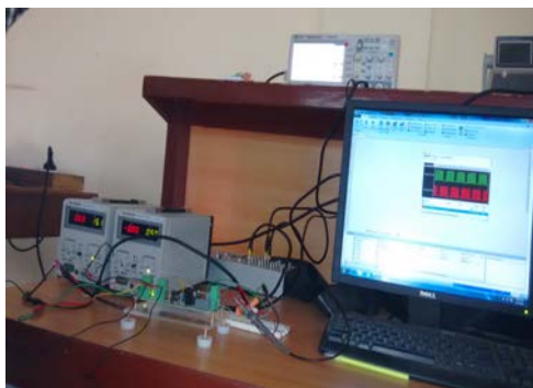
Fig. 7 Testing of circuit in dSPACE DS1104
